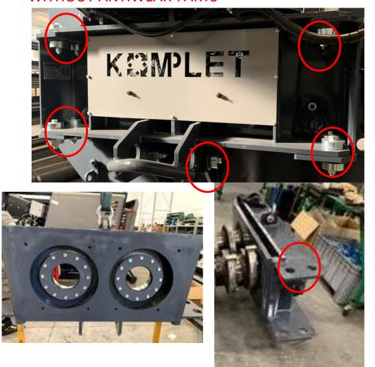
SHAFTS SUPPORT WITH LEES BOLTS TO FIX AND WITHOUT ANTIWEAR-PARTS
