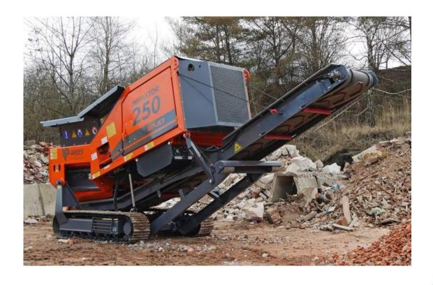
Discharge height (mm) 3.400 Width (mm) 800
