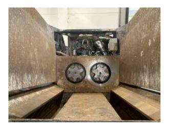
THE GRANGLOMETRY OF MATERIAL IS SETTING BY THE SIDE WALL GRID THAT CAN WORK CLOSE (to have serial from 0 to 100/150 AND CAN WORK DIFFERENT MATERIAL LIKE WOOD OR PLASTIC
