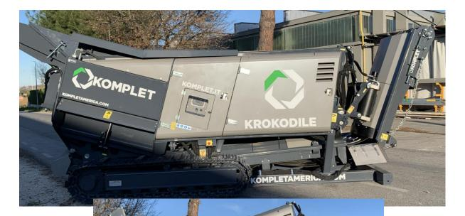
The machine can be drive by undercarrige or by hooklift (to load by hook lift if have a rear tilt hopper should be dismantle in some country depending on internal legisaltion)
