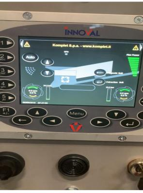
\COMPUTER ON BOARD MENAGE THE RPM OF SHAFT AND ALSO COMUNICATE WITH HYDRAULIC SYSTEM TO HAVE REVERSE AND DIFFERENT RPM OF ROTATION OF SHAFTS
